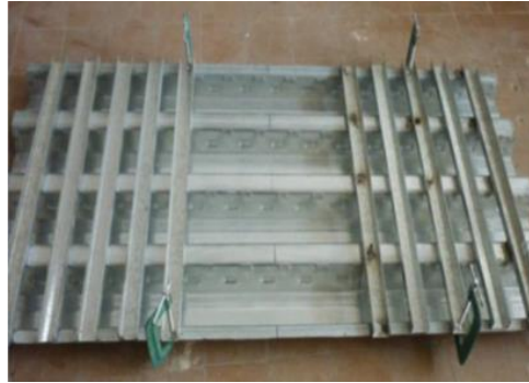
Fig.6 (b) Cold-formed members as shear connectors
