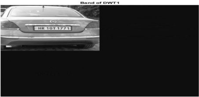
Fig.3 Wavelet transforms performed on the greyscale image, representing LL, LH, HL, and HH sub-bands.
