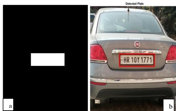
Fig 7 a) Unwanted regions are eroded by Morphological operation, final LP region is retained. b) Final Plate region
