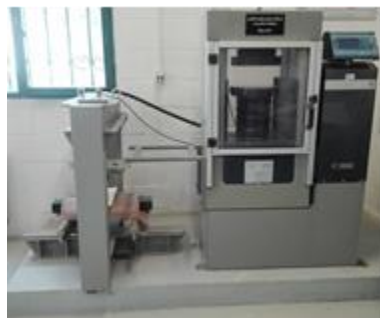
Figure 1-bending and compression strength test device [Writer]
