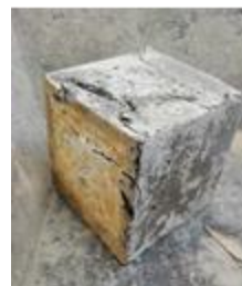
Figure 2- Pressure samples and a sample of broken compression sample [Writer]
