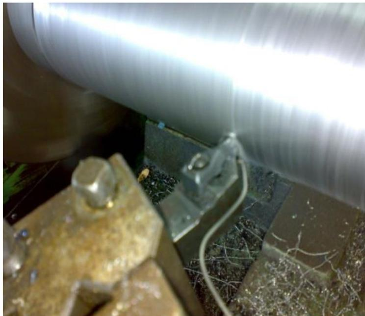
**Fig. 3** Actual tool temperature measurement showing thermocouple wire and holder
