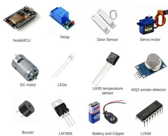
Fig 3.5: Components used in hardware implementation
