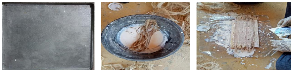
Figure 2. Mould, latex immersion and stacking of fibers
