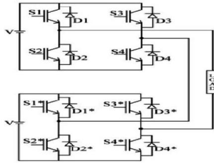
**Fig.3 Structure of a single-phase H-bridge inverter with many levels of cascaded H-bridges**
