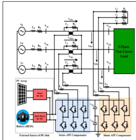
**Fig.1. UPQC system configuration**
