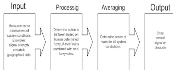
**Fig.4. The FUZZY logic Control-Analysis method**
