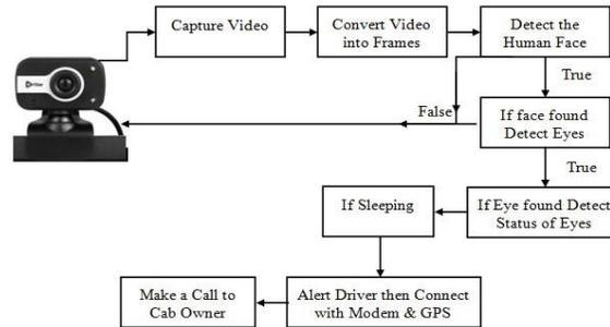
Figure 1 System Architecture
