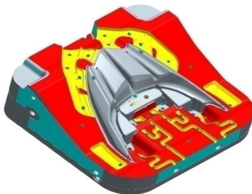
Fig.11. Insert on which cluster plate machining and sparking is performed
