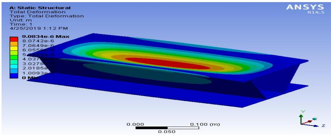
**Figure 7(a).** Total deformation for case 2
