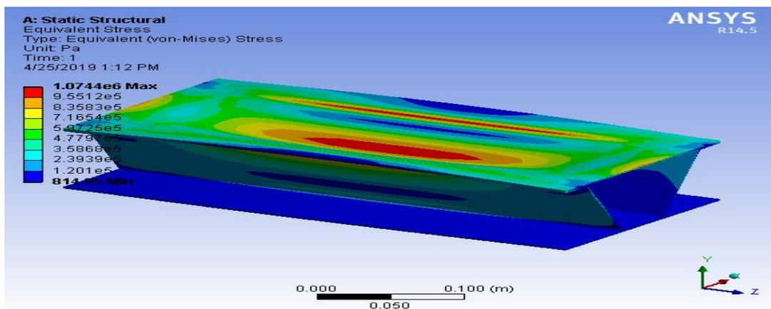
**Figure 7(b).** Von-Mises stress for case 2
