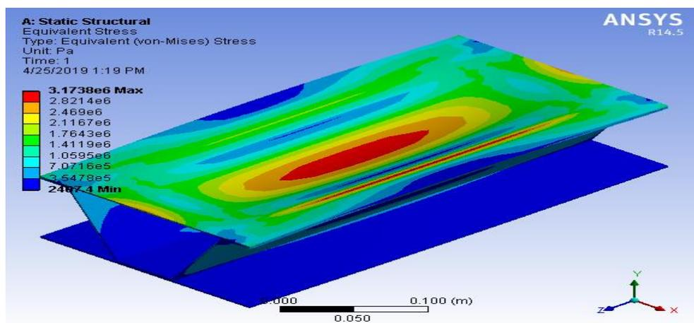
*Figure 9(b). Von-Mises stress for case 4*
