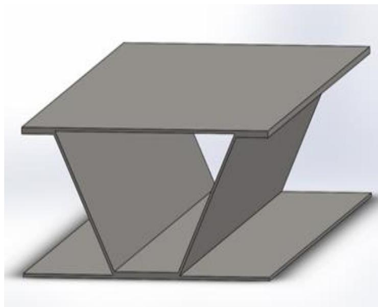
*Figure 5. Geometry of Corrugated core sandwich panel*
