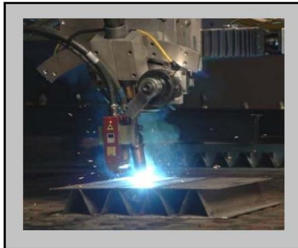
*Figure 3. Laser Welding Of Corrugated core.*
