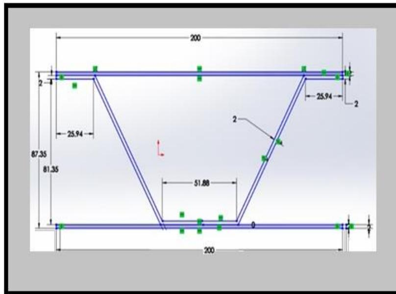
*Figure 2(b) . Dimensions of a corrugated core*
