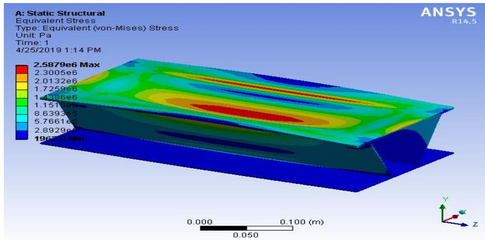
*Figure 8(b). Von-Mises stress for case 3*
