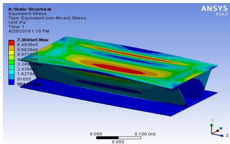
Figure 6(b). Case-1 Von-Mises stress for case 1
