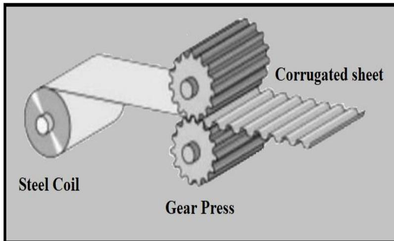
*Figure 1(a) Mechanical Rolling Pressing tool*
