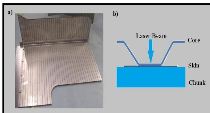
*Figure 4 Welding of Skin with core*
