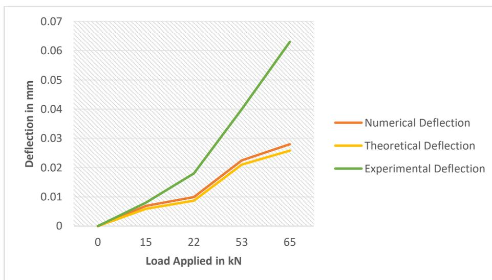
**Figure 10:** Comparison Of Numerical, Theoretical and experimental results
