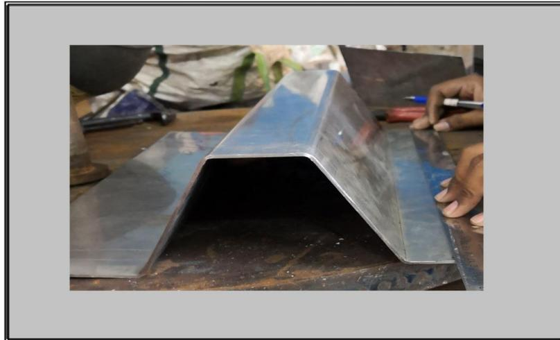
*Figure 2(a) . Corrugated core made by Press Tool*
