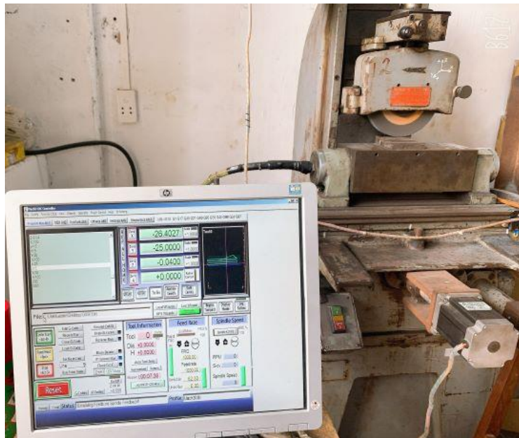
Fig 4.2. Automatic grinding with the program loaded on the NSG-550B machine
