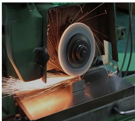
Fig. 1.1. The machining on the flat grinding machine tool
