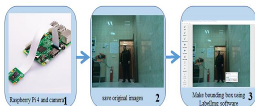
Fig. 2. The proposed block diagram of dataset processing.
