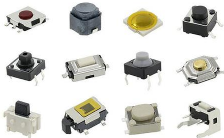
Figure 10. Types of switches and pushbuttons
