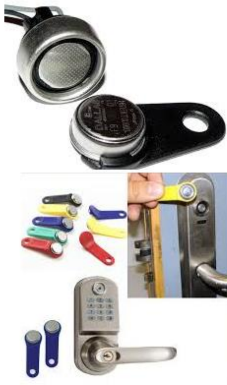
Figure 2. iButton and Secure Lock using iButton.
